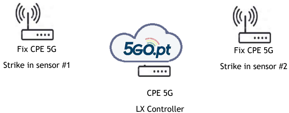
Figure 8 – Safety Critical scenario communication - the strike in sensors send strike in message to the LX controller when detects the approaching train
