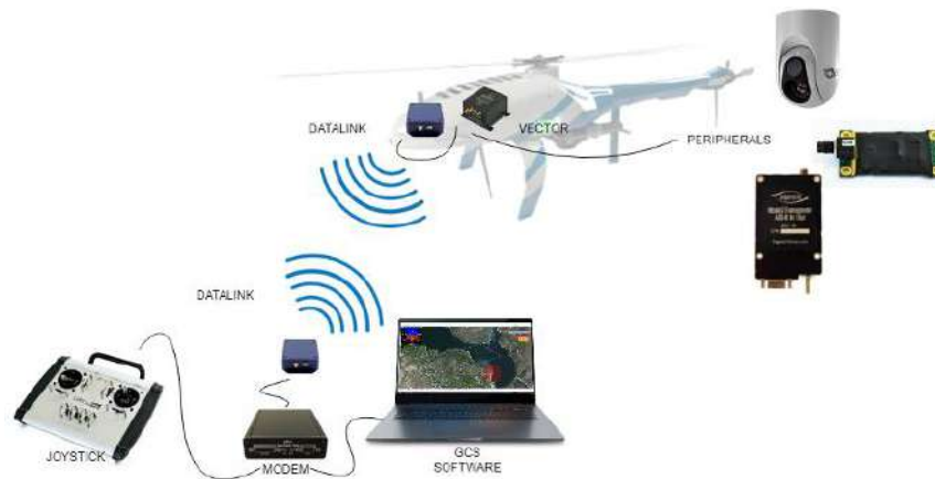
Figure 1 – UAV Navigation communication setup 7
